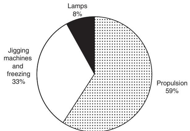
**FIGURE 5** Functional fuel utilization on a Japanese long-distance squid fishing vessel. Data from Ishikawa, *et al.* (1987). A case study of energy analysis of long distance squid angling. *Bull. Jap. Soc. Sci. Fish.* 53(9), 1525–1531.
